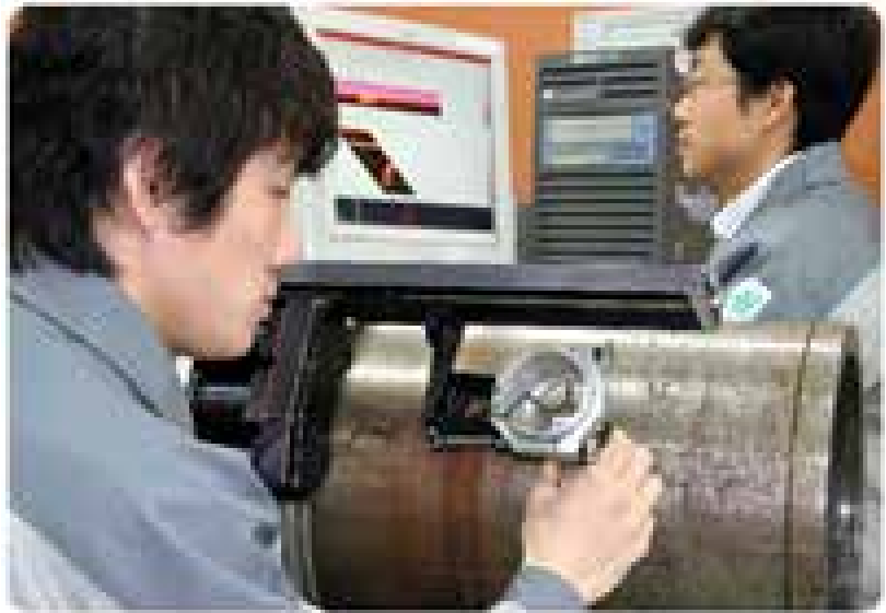
Inspection Services for Piping, Equipment, and Structures (UT)
